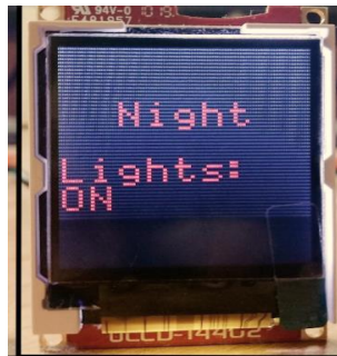
Figure 24: Example of Light Intensity Sensor Output
