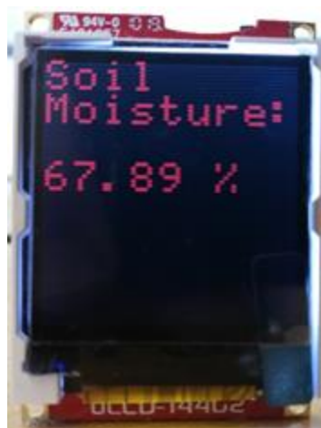
Figure 28: Soil moisture displayed on the uLCD screen
