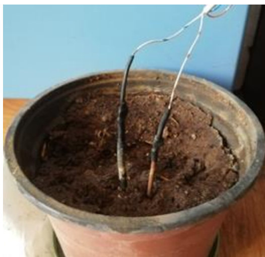
Figure 26: Soil Humidity Experimental Setup
