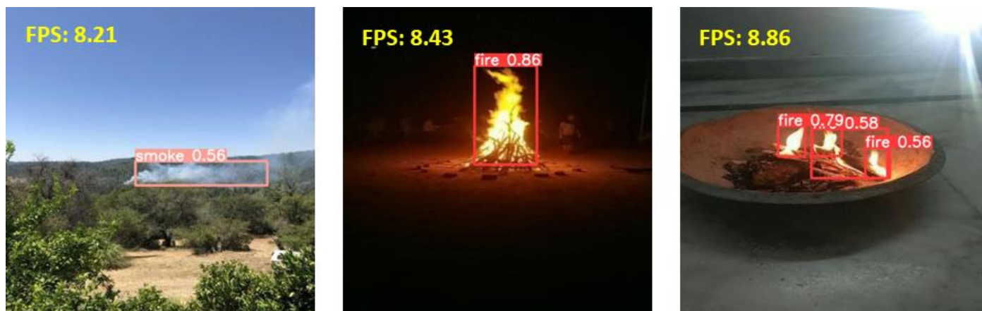
Figure 50: Detection Results on Raspberry Pi Platform
