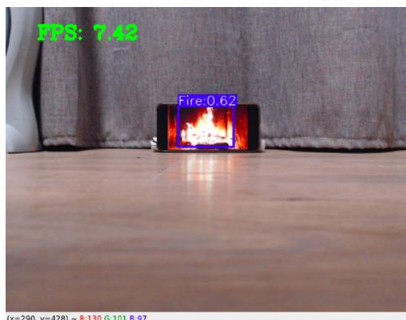
Figure 54: 1080p HD quality at over 7FPS on the Raspberry Pi 4B
