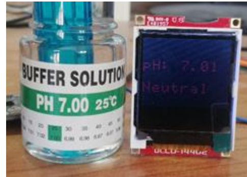
Figure 14: Example of Display Message with pH = 7
