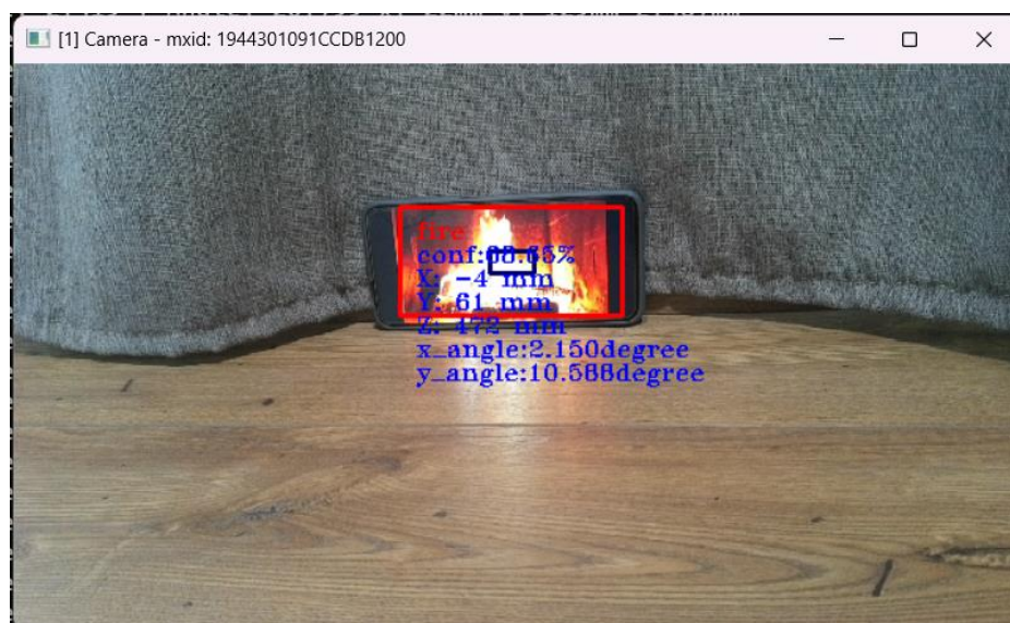
Figure 105: Obtaining the distance, angle offset and other information using the proposed system.
