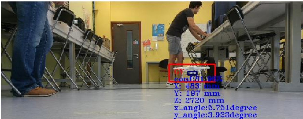
Figure 113: UAV Placed on a box to Verify Altitude Calculations
