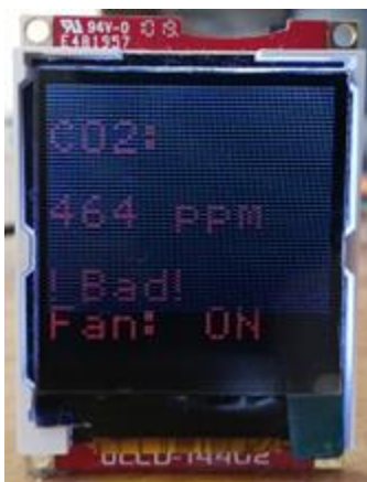
Figure 19: ppm value displayed on the uLCD screen
