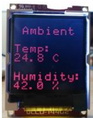
Figure 5: Ambient (Outside) Temperature & Humidity displayed on the uLCD screen
