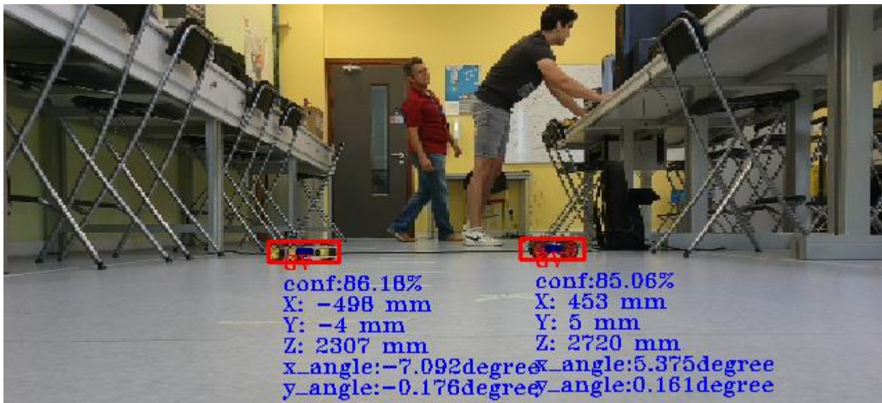
Figure 115: Profile Camera Detecting 2 UGV Simultaneously
