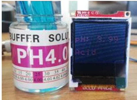
Figure 13: Example of Display Message with pH = 4
