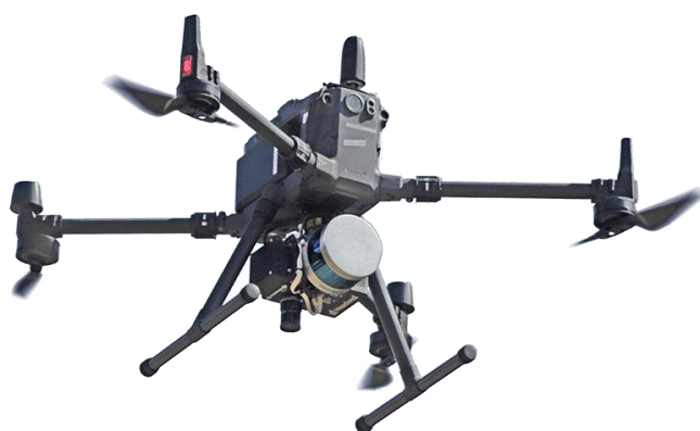
Figure 32: Nano HP (400-1000nm) Hyperspectral Imaging Package [5]
